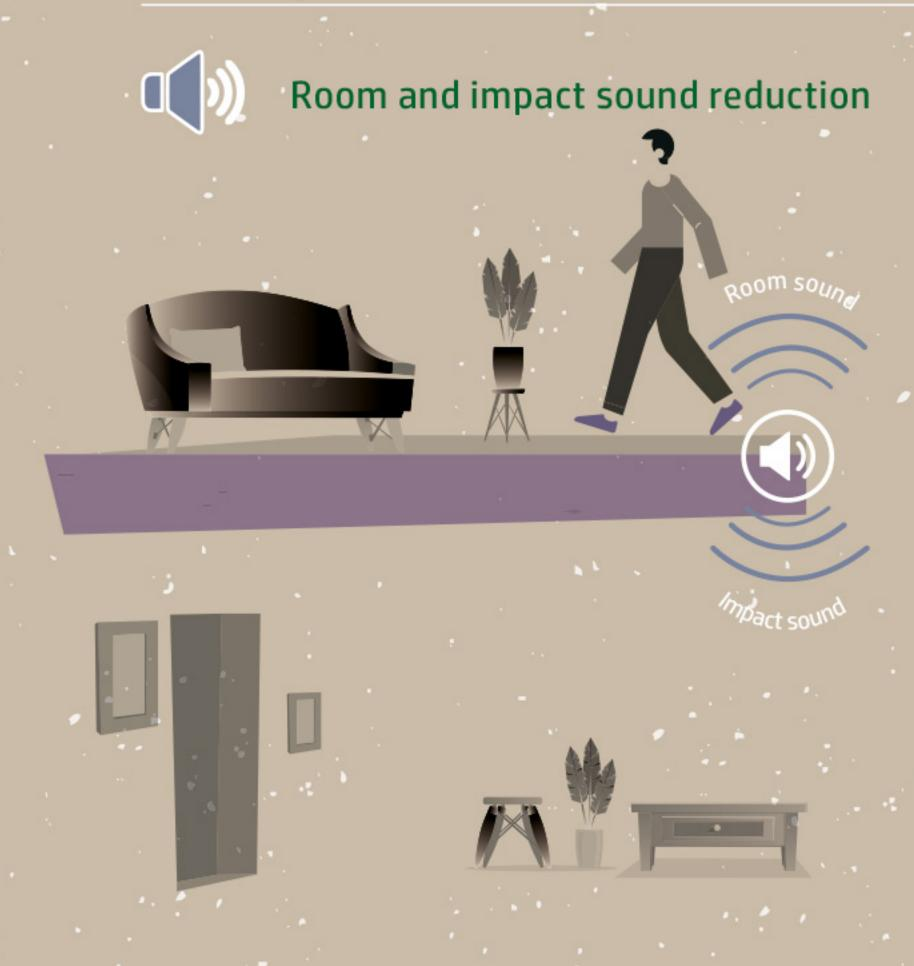
The 8 - 10 mm total HDF thickness and the cork backing ensure reduced room and footfall noise.
